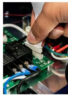
**3.** Once the top portion of the control module has been lifted you can now see the three wires that are inserted into the cell connection housing. Using your hand, apply slight pressure to the wires that are associated with the out-of-place metal prongs back into the cell connection housing until you hear a click noise.
