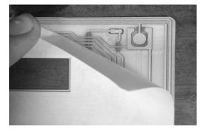
9. Place the green/black ribbon cables through the provided slot, and then press the new keypad onto the blue surface area.
