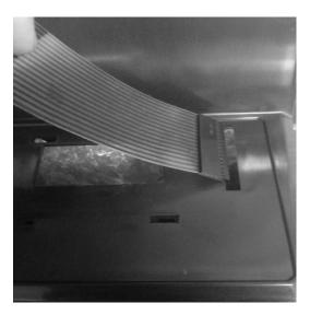
10. Reconnect the black/green ribbon cable back to <u>both</u> terminals on the Display circuit board. **If your keypad utilizes a RJNK16 keypad (11/9 pins)**, align outer cable towards end marked "R7"; this should leave open "R15" & "R16" near "Key"
