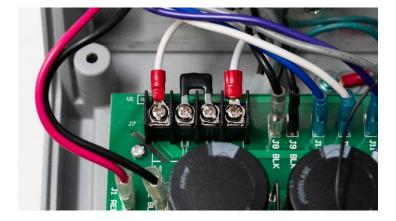
3) Loosen all four screw terminals, remove wires, and remove the existing jumper.
