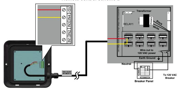
IN4 It is controlled by a relay of the external controller. After the relay is closed, four kinds of speeds can be realized corresponding to different running times. The time and speed are all completed on the pump operation panel. Refer to the Programming a Custom Schedule 1-14 for the specific operation steps (in the SmartFlo pump's manual).
