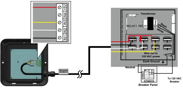
IN1/IN2/IN3 is controlled by external relays. After the relay is opened and closed, the running time corresponding to the speed can be realized. The speed is completed on the
