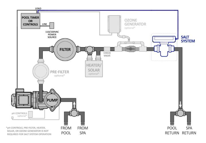
The **CORE**-SERIES consists of one assembly that incorporates all of the following: Control Module, Electrolytic Cell, Flow Switch, and Temperature Sensor.
