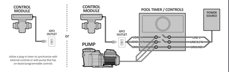
If a hardwire connection is desired, the wiring can be modified by a qualified person.
